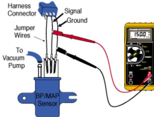
**Fig 8 - Using DC-Coupled Hz to Check BP/MAP Sensors** To test the performance of a BP/MAP sensor, graph its frequency output at various levels of vacuum. Start with the sensor at 0" Hg (0 cm /hg) and read its frequency. Then note the frequency at each increase of 1" Hg (cm Hg). When you plot these frequencies, they should be in a straight line. The frequency will decrease with an increase in vacuum.
