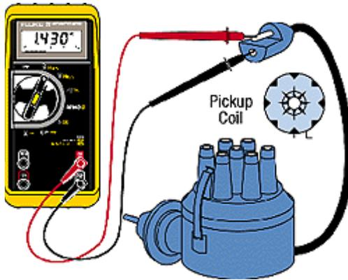
**Fig 15 - Checking For Pulses from Magnetic Distributor Pickup** Disconnect the distributor from the ignition module. Connect the DMM across the pickup and set it to AC volts. When the engine is cranked, pulses should appear on the bar graph. If no pulses appear, it is likely the reluctor wheel or the magnetic pickup is faulty. Use this technique for other magnetic position sensors too. On GM cars, remove the distributor cap for access.
