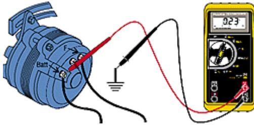
**Fig 4 - Checking Ripple Voltage** Ripple voltage or (AC voltage) can be measured by switching your DMM to AC and connecting the black lead to a good ground and the red lead to the "BAT" terminal on the back of the alternator, (not at the battery). A good alternator should measure less than .5 VAC with the engine running. A higher reading indicates damaged alternator diodes.
