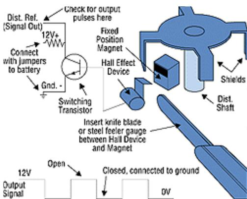
**Fig 14 - Checking Hall-Effect Sensors** Check for reference voltage from battery at connector. Hall sensors require power where magnetic sensors do not. To test sensor: connect +12V from battery to power terminal, set DMM to measure volts and connect it between signal output and ground. Insert feeler blade between sensor and magnet while watching for the bar graph to move. Signal should vary from 12V to 0V.
