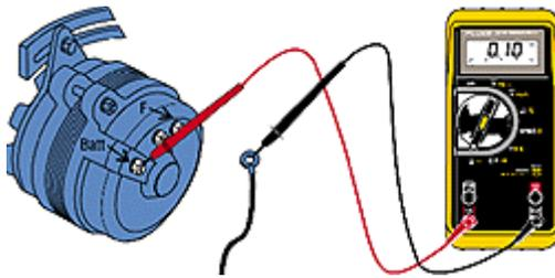
**Fig 5 - Alternator Leakage Current** To check alternator diode leakage, connect the multimeter in series with the alternator output terminal when the car is not running. Leakage current should be a couple of milliamps at most; more often, it will be on the order of 0.5 milliamps. Use care when disconnecting the alternator output wire; make sure the battery is disconnected first.
