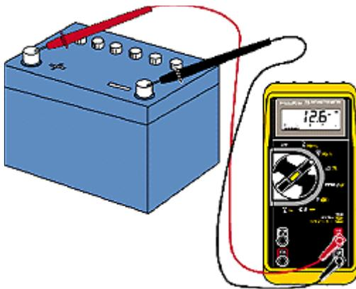
**Fig 1 - Measuring System Voltage** Bleed the surface charge from the battery by turning on the headlights for a minute. Measure the voltage across the battery terminals with the lights off (see chart). When possible, individual cell specific gravity should be checked with a hydrometer. A load test should be done to indicate battery performance under load. Voltage tests
