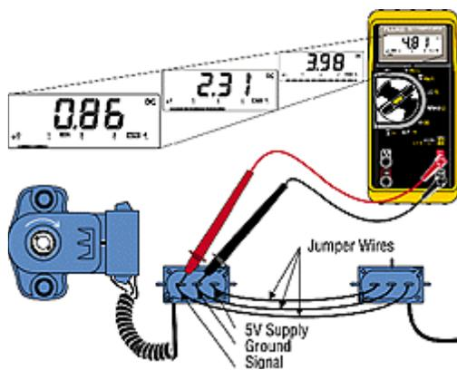
**Fig 11 - Testing a Throttle Position Sensor** Use the Min/Max recording feature of the Fluke 78 to check your base TPS setting at idle; to get the maximum reading, depress the accelerator. By comparing these readings to those you get when you open the throttle by hand, you can verify whether the throttle cable and/or linkage is properly adjusted to allow full throttle opening. If it isn't, this may be the source of a problem with poor acceleration.
