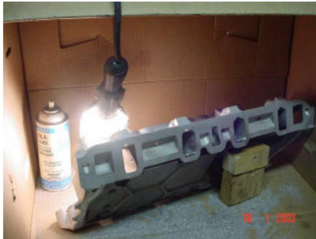
Notice I use blocks of wood for holding the intake in a good position for porting the runner I'm working on. Also notice the silicone lubricant that I spray lightly on the burr every couple of minutes to keep the burr from loading up with slivers. I use carbide bits, which are normally used for steel, I like to use them because they don't remove material as fast, they really allow me to shape the cut, and they leave a very smooth cut on the wall.
