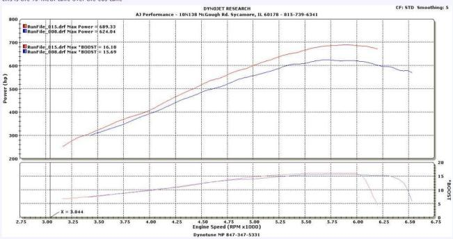
92 GT. FORDSTROKERS 363 ,forged crank rods, custom 9:1 pistons, custom freezy74 cam, innovators zero balancer w/ crank trigger, TW 205's, 1.7 HS shafts, tfs box r port matched, 90mm tb, 97mm dbx, andersom power pipe, si-trim , tremec , 3.73, meth injected. and lots more. 689rwhp. FORDSTROKERS IS WHERE ITS AT!!!
